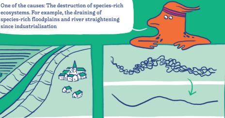
Straightened and deepened rivers enabled the use of heavy transport ships. Gravel and shallow banks were lost as habitats and the groundwater level sank.
